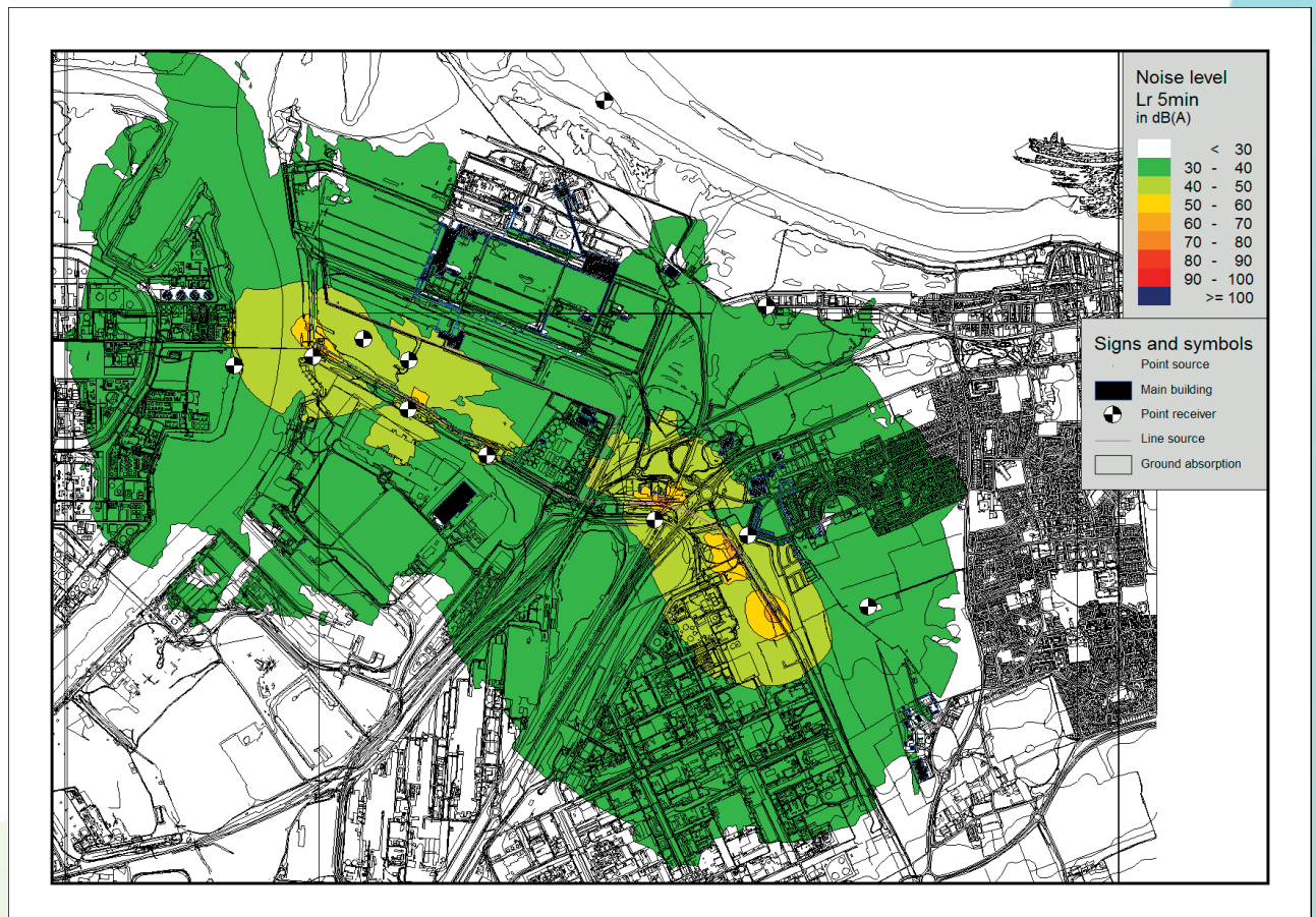
Figure 9-6 Noise contour plot of mitigated quay percussive piling and south conveyor construction piling
